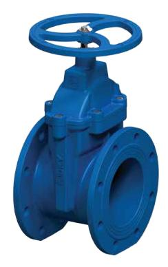
Resilient Seated Gate Valves are used for general purpose on/off operations in municipal, agricultural and industrial infrastructural networks. The sealing is achieved by the vulcanized rubber on the wedge acting directly on the body internal wall.
